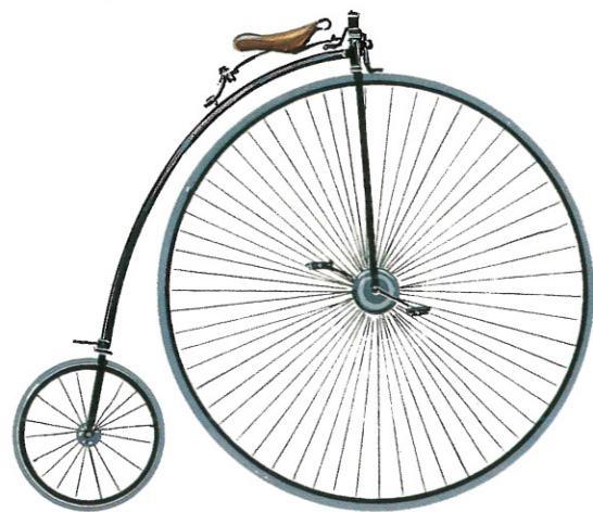
The first bicycles were uncomfortable and dangerous. The "penny farthing" was invented by James Starley in the early 1870s, and had solid tires and no brakes.
